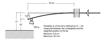
Figure 8. Foil dimensions and flexibility
