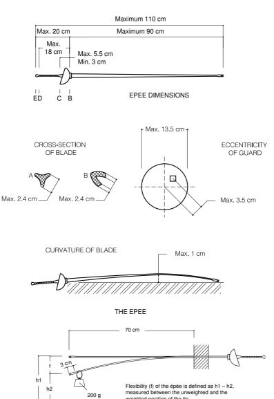
Figure 9. Epée dimensions and flexibility
