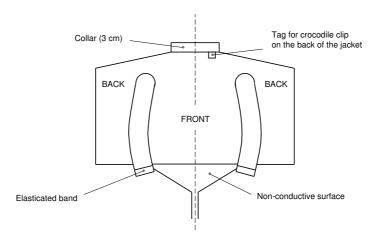
Figure 15. Electric sabre: conductive jacket
